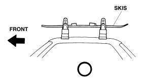
9. If the bindings cannot be positioned between the front and the rear attachments, install the skis with the rear bindings behind the rear attachment as shown.
